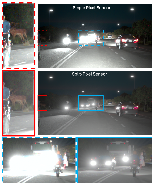
Fig. 7. A split pixel 3-capture sensor and flare. We used the scene in Figure 5 to simulate the 3-capture split pixel image. The data from the single pixel, large photodetector sensor are saturated over large regions, due to lens flare (top). The small photodetector data preserve image contrast in parts of the image that are saturated by flare, and thus the combined image enhances the visibility of the motor cyclist (solid blue boxes) compared to the single pixel (dashed blue boxes). The combined image retains the visibility of the deer in the dark image region (red boxes).
