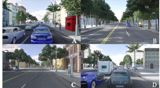
Figure 3. Scenes generated on the same road and sky map, but randomly sampling buildings, trees, environmental objects and setting different traffic and environmental parameters. (A,D) High traffic density. (B,C) Low traffic density. The camera position is chosen to be consistent with the car that is acquiring the image (not shown).
