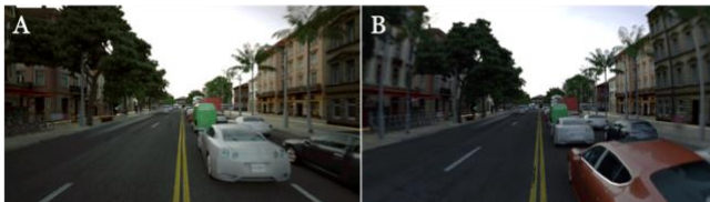
Figure 5. A comparison of cameras with different imaging lenses. (A): wide angle lens; (B): fisheye lens
