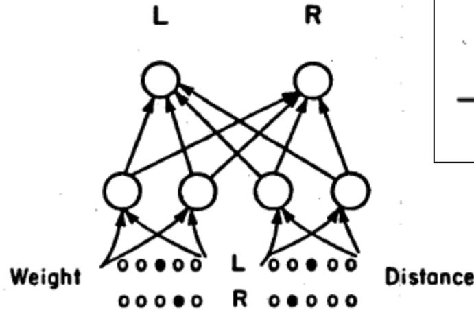
**Input units** for number of weights and distance on each side of a balance
