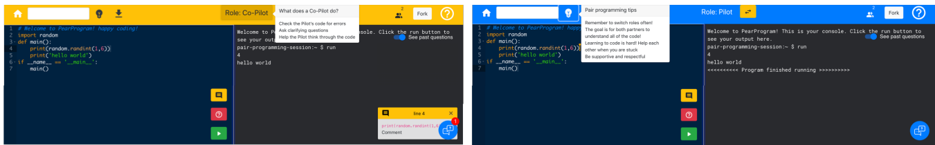
Figure 1: An example PearProgram session as seen from the copilot view (yellow) and pilot view (blue). The left-hand panel of the application is a text editor and the right is where the code output appears. The white text boxes at the top of each screen are some of the tips for pair programming embedded within the tool.
