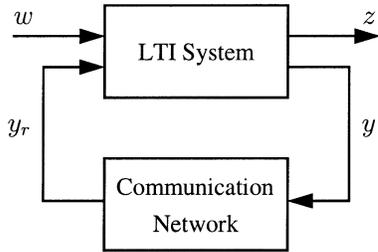
Fig. 1. Linear time-invariant (LTI) system closed over communication network.
