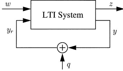
Fig. 4. Additive-white-noise model for quantization errors.
