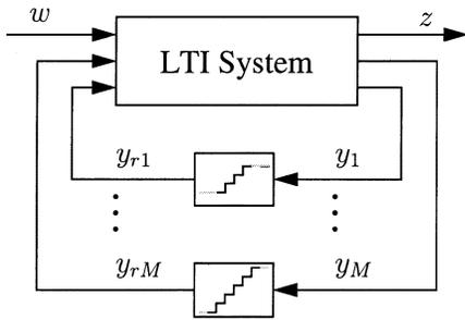
Fig. 2. Uniform quantization model of communication links.
