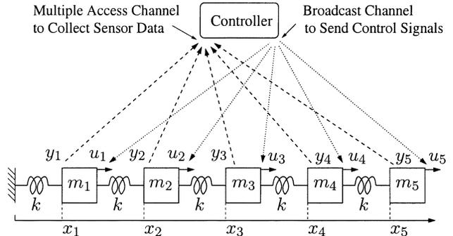
Fig. 6. Control of a mass-spring system.
