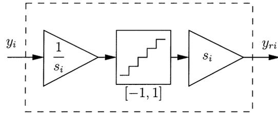
Fig. 3. Scaling of the uniform quantizer.
