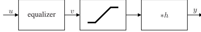
Fig. 5: Our pre-equalizer processes the incoming signal u (with a look-ahead of T samples) to produce the input v applied to the system.
