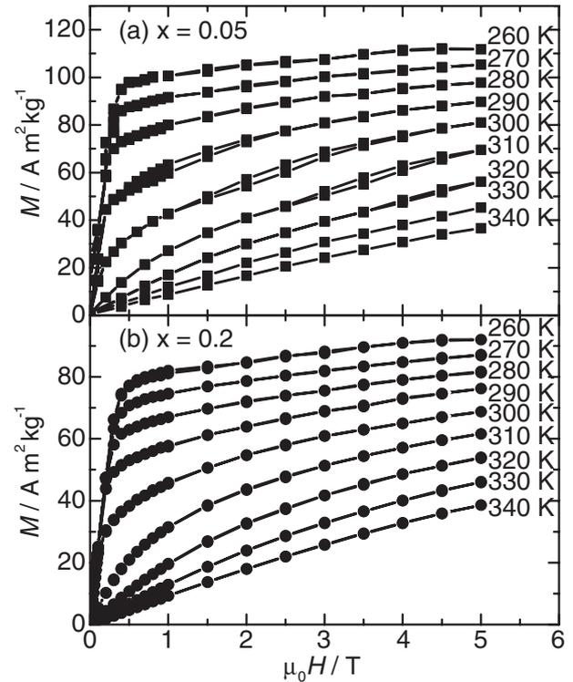
Fig. 2 Magnetic field dependence of the magnetic moment  $M$  at various temperatures for (a)  $x = 0.05$  and (b)  $x = 0.2$  around  $T_C$ .
