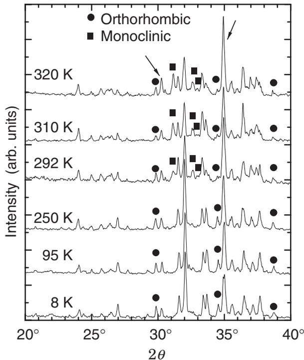
Fig. 4 Powder X-ray diffraction patterns of  $\text{Gd}_5(\text{Ge}_{1.8}\text{Fe}_{0.2})\text{Si}_2$  at various temperatures. The solid squares and the circles denote the characteristic peaks of the monoclinic and orthorhombic phases, respectively. Arrows indicate the diffraction peaks of the minor phase.
