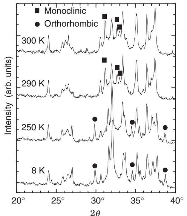
Fig. 3 Powder X-ray diffraction patterns of  $\text{Gd}_5(\text{Ge}_{1.95}\text{Fe}_{0.05})\text{Si}_2$  at various temperatures. The solid squares and the circles denote the characteristic peaks of the monoclinic and the orthorhombic phases, respectively.
