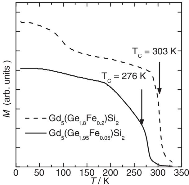
Fig. 1 Temperature dependence of the magnetic moment of  $\text{Gd}_5(\text{Ge}_{2-x}\text{Fe}_x)\text{Si}_2$  for  $x = 0.05$  (solid line) and  $x = 0.2$  (dashed line) in magnetic fields of 0.1 T. Arrows indicate the Curie temperatures.
