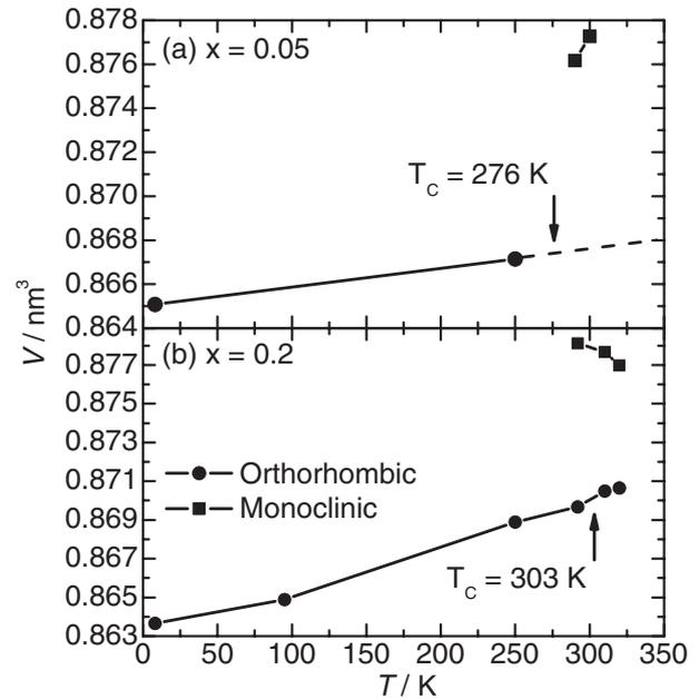
Fig. 5 Temperature dependence of the unit cell volume  $V$  of  $\text{Gd}_5(\text{Ge}_{2-x}\text{Fe}_x)\text{Si}_2$  for (a)  $x = 0.05$  and (b)  $x = 0.2$ . The solid squares and the circles denote the volumes of the monoclinic and orthorhombic phases, respectively.
