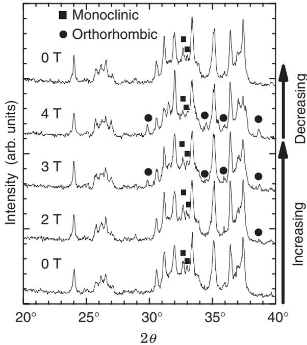
Fig. 6 Field dependence of the powder X-ray diffraction patterns of  $\text{Gd}_5(\text{Ge}_{1.95}\text{Fe}_{0.05})\text{Si}_2$  at 290 K. The solid circles and the squares denote the characteristic peaks of the orthorhombic and the monoclinic phases, respectively.
