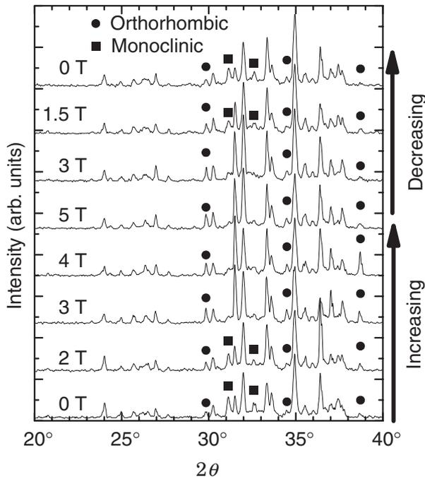
Fig. 7 Field dependence of the powder X-ray diffraction patterns of  $\text{Gd}_5(\text{Ge}_{1.8}\text{Fe}_{0.2})\text{Si}_2$  at 310 K. The solid circles and the squares denote the characteristic peaks of the orthorhombic and the monoclinic phases, respectively.
