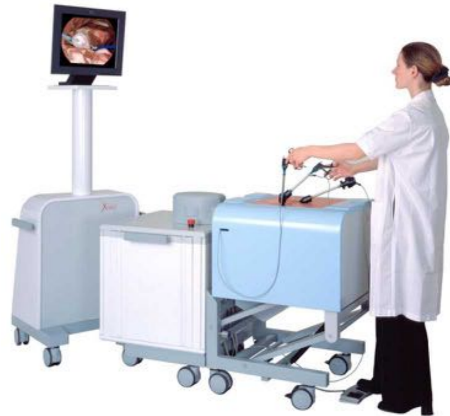
Laparoscopic Simulator with haptic feedback (Launay, Xitact, Switzerland)
