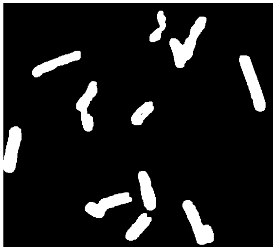
dilation with 3x3 structuring element
