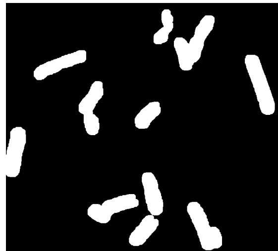
dilation with 7x7 structuring element
