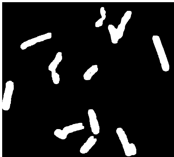
dilation with 3x3 structuring element
