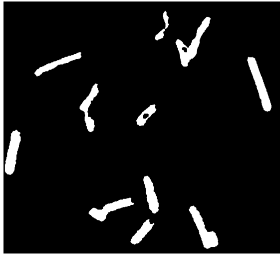
erosion with 3x3 structuring element
