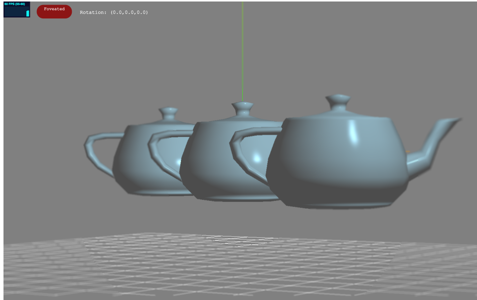
Figure 6: Foveated rendering. Here is something you might see when you implement the foveated rendering. Please note that this is exaggerated, and the actual blurs you will implement will be much more subtle. This is just so you can see the effect of the of the different regions in this document.
