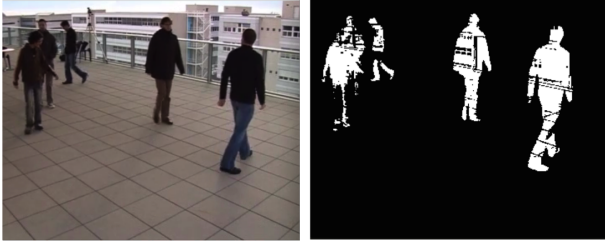
Figure 5: Example of applying background subtraction on one frame of a video.
