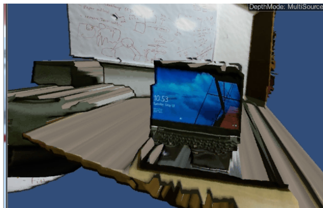
Figure 7: Live feed of Kinect depth & RGB values, reconstructed into a dynamic mesh in Unity. Note the phantom surface artifacting at the sides of objects where the Kinect could not capture depth information.
