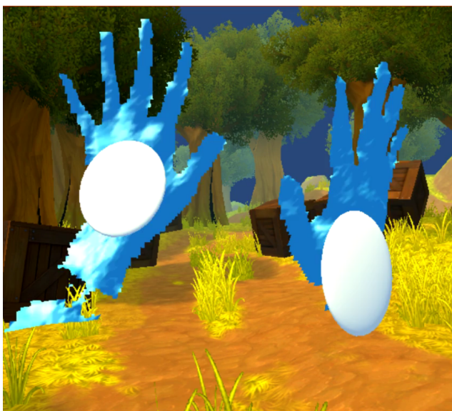
Figure 9: Real-time hand tracking in VR. The white discs attached to the hand are an estimate of the hands' centers. This is a screenshot of a live scene rendered in Unity
