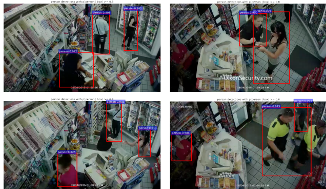
Figure 4. Example bounding box predictions for the retail video data. These were generated without doing image distortion correction, although in our final implementation we were sure to correct distortion first if it was present.
