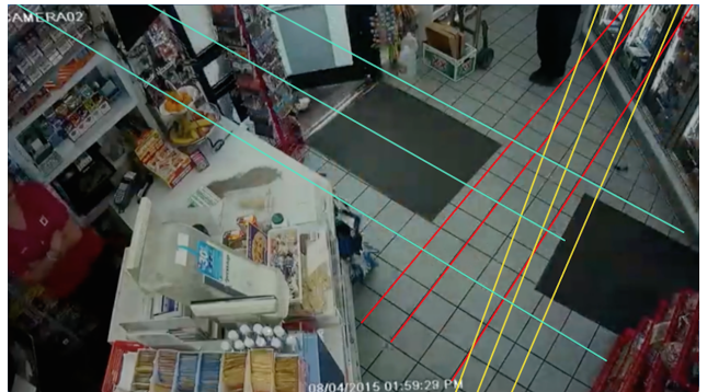
Figure 1. Sets of mutually orthogonal lines used for single view metrology calibration in the retail camera frame. The line intersections give us three vanishing points, which we use in the equations above to solve for K.
