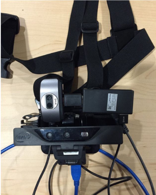
Figure 2. Chest-mounted egocentric camera setup with both RGB-T and RGB-D cameras attached to a GoPro chest harness
