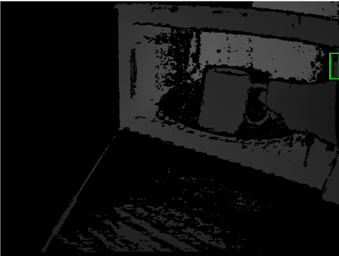
Figure 14. An example of a mistaken hand detection for the depth video data
