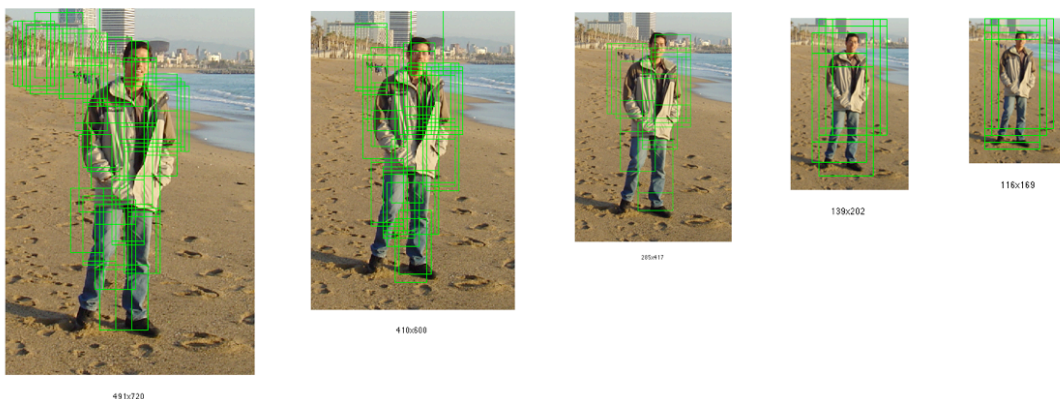
Figure 3: exhaustive search using sliding window over a pyramid of scaled images, using SVM classifier
