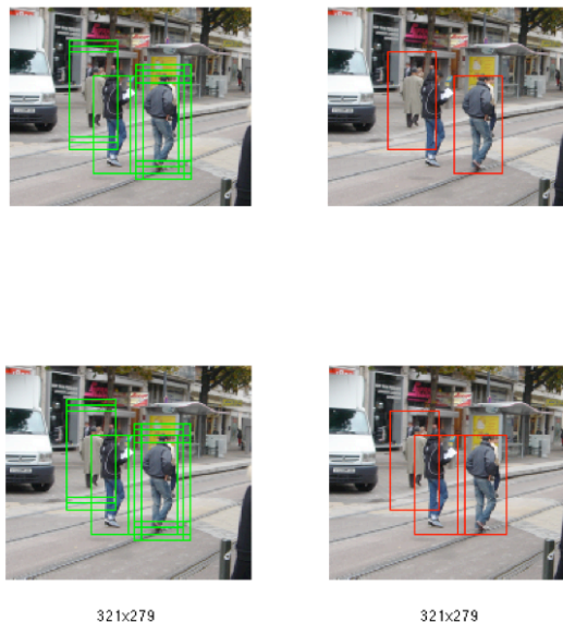
Figure 4: non max suppression with different window sizes, when looking for local maximum of weight cost.
