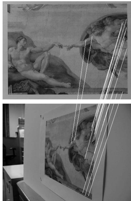
Figure 1. Typical case of failure of SIFT due to very different viewpoints : only 15 matches are found. Credit : J.M. Morel, G. Yu , ASIFT: A New Framework for Fully Affine Invariant Image Comparison
