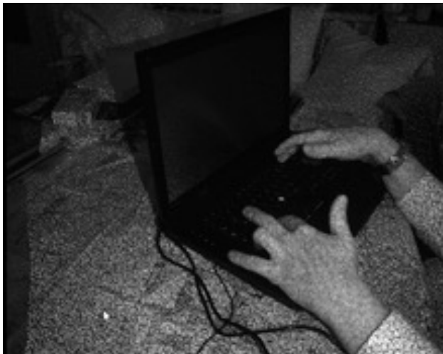
Pattern of projected infrared points to generate a dense 3D image
