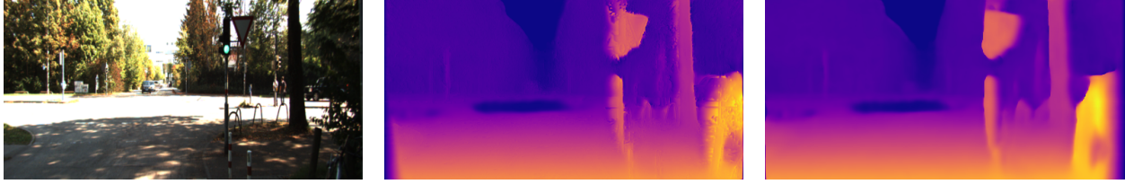
Figure 3: Input and output (left/right disparity) of trained monocular depth estimation networks.
