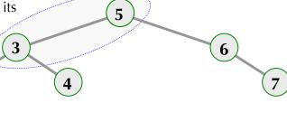
one level closer to the root, the former parent of 5 becomes 5's left child and in the process inherits what **used** to be the left child of 5 as its right child. In general, these two nodes might occur anywhere in a binary search tree. Notice that the binary search tree property is maintained.
