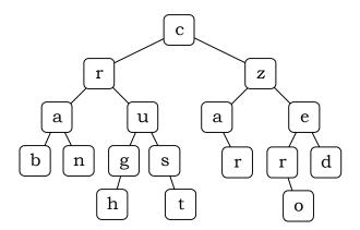
should be able to confirm that presence of words like "crab", "ran", "rug", "crust", "rust", "us", "ugh", "czar", "zero", and "zed". "rug" and "us" are noteworthy, because they neither start at the root nor end along the fringe—they're completely internal. ("arc" doesn't count, because it's going the wrong way.)
