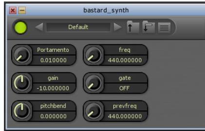
Figure 1: VST plug-in generated by Faust as it appears in MuLab. Using predefined control names “freq”, “gain” and “gate” automatically maps the controls to MIDI event parameters.
