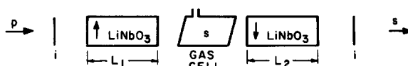
Fig. 1. Schematic of frequency locking technique. The letters s , i , and p denote the signal, idler, and pump, respectively. The gas transition is assumed to absorb at only the signal frequency; and the mirrors are assumed to have high reflectivity at only the idler frequency. The vertical arrows in the \text{LiNbO}_3 crystals denote the direction of their positive z axes.
