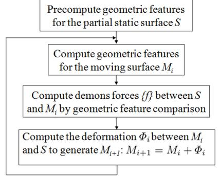
Figure 2: Thin Shell Demons workflow.
