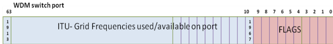
Figure 2.7: Representing bandwidth in WDM switches
