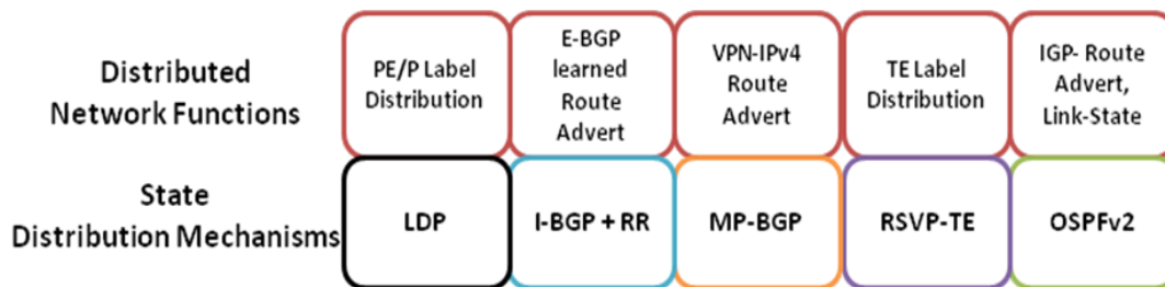
Fig. 5.6 Network Functions in Today's IP/MPLS Networks
