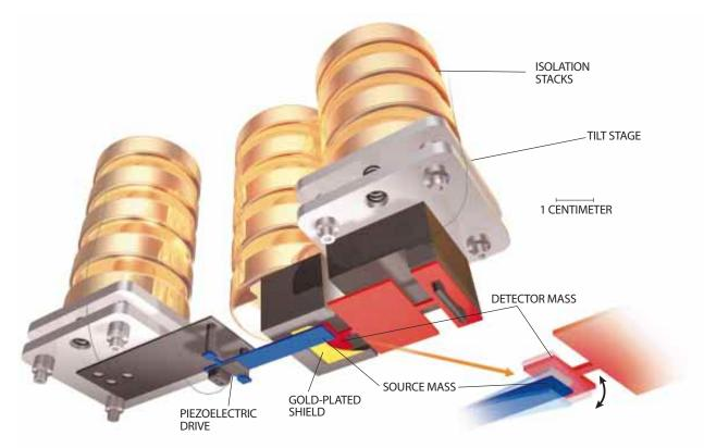
**TORSION OSCILLATOR** at the University of Colorado looks for changes in gravity from 0.05 to 1.0 millimeter. Piezoelectrics vibrate the tungsten source mass (*blue*) like a diving board. Any forces acting between the source mass and the tungsten detector (*red*) produce twisting oscillations of the detector (*inset; oscillations are exaggerated*), which are sensed by electronics. A gold-
