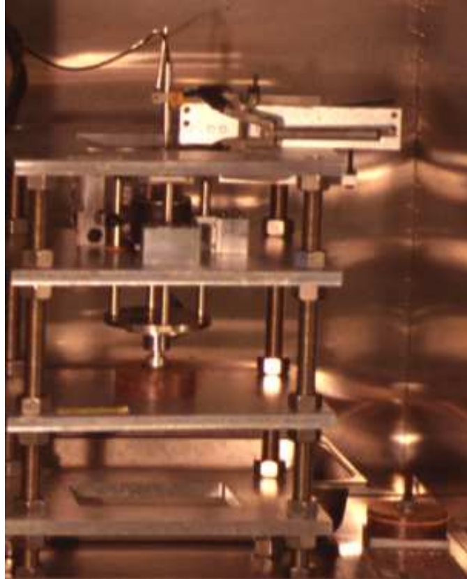
Figure A-2: The incustat machine inside a standard cell culture incubator. The chamber in the machine is being compressed. The chamber to the right of the incustat is being used as a static control.
