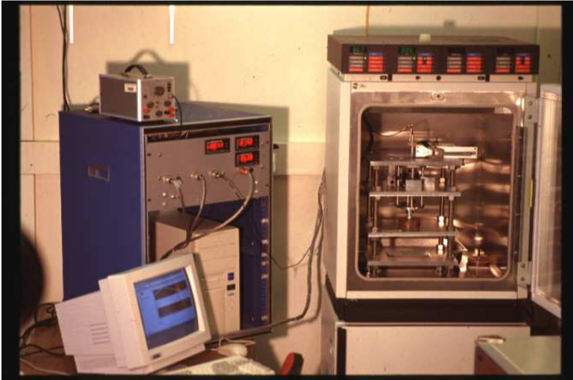
Figure A-6: The incustat within its incubator along with the controlling computer and electronic hardware. This is an old picture taken when an actual signal generator was used to drive the hardware feedback circuitry in dynamic compression experiments.
