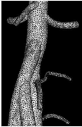
Fig. 7. Close-up of finite element mesh for aorto-femoral bypass with end-to-side anastomosis.
