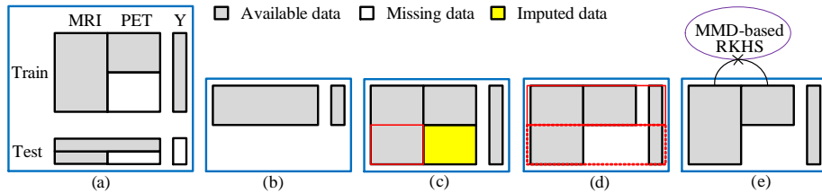
Fig. 1. (a) Block-wise incomplete multimodality data, (b) Disposal method, (c) Imputation method, (d) Multi-task learning method, and (e) Proposed method, which nonlinearly maps heterogeneous MRI and PET data into a common RKHS so that they are comparable, and thus allowing to learn a common MKL-based classifier.
