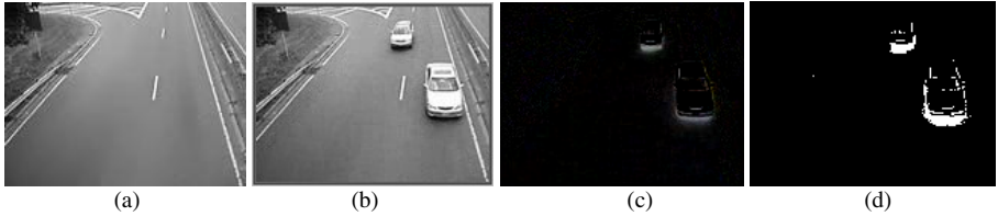
Fig. 4. (a) Extracted background image. (b) A sample frame of the video sequence. (c) Background subtraction, subtracting frame image from the background. (d) Binary Image of c.
