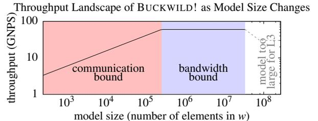
Figure 2: Bounds for throughput as model size changes. Dashed line represents the setting where the model is too large to fit in the L3 cache.
