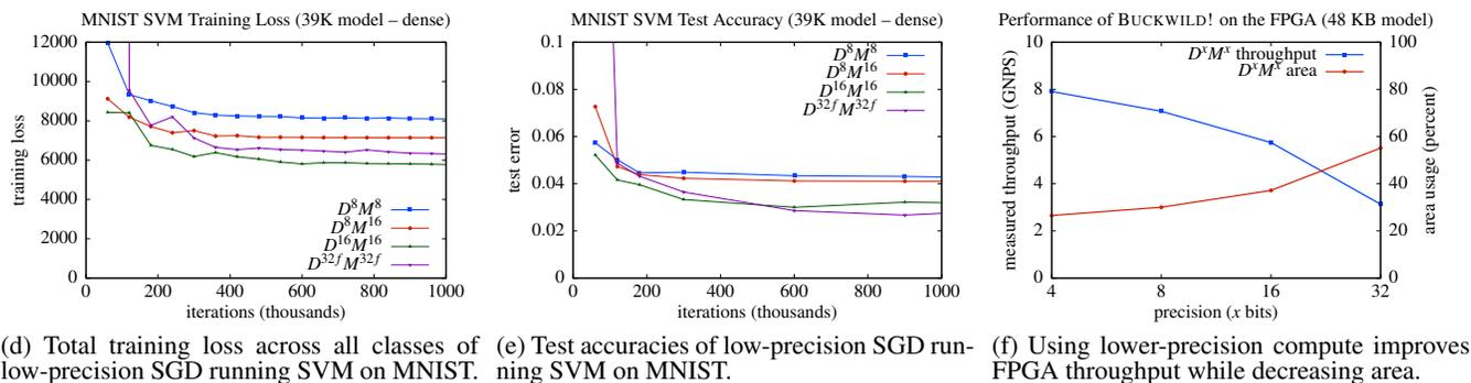
(d) Total training loss across all classes of low-precision SGD running SVM on MNIST. (e) Test accuracies of low-precision SGD running SVM on MNIST. (f) Using lower-precision compute improves FPGA throughput while decreasing area.
