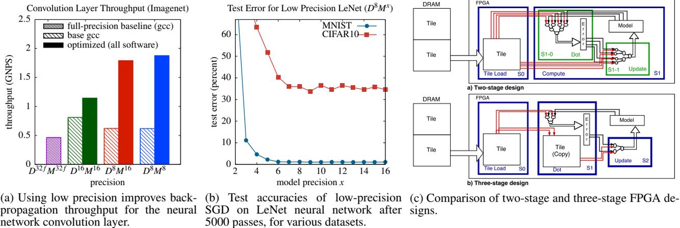
(a) Using low precision improves back-propagation throughput for the neural network convolution layer. (b) Test accuracies of low-precision SGD on LeNet neural network after 5000 passes, for various datasets. (c) Comparison of two-stage and three-stage FPGA designs.
