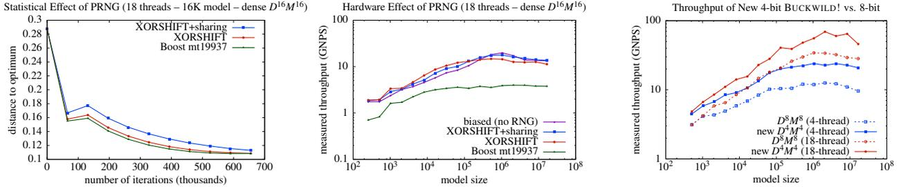
(a) Statistical efficiency comparison of multiple random number generation schemes, each averaged over 5 runs (dense SGD). (b) Hardware efficiency comparison of multiple random number generation schemes (dense SGD). (c) Adding instructions to enable 4-bit computation improves throughput by up to a factor of 2.
