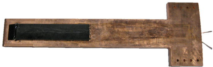
Figure 4. Fuel, Support and Ignition. The fuel grain is epoxied to the copper support. A nichrome wire is placed just behind the chamfer at the fore end. It is coated with epoxy to ignite the fuel. Lead wires run under the support and out the aft end of the combustion chamber.
