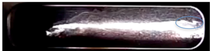
Figure 14. HTPB. The flame from the HTPB run. Flow structure is clearly visible at the aft end. The flame is much brighter than the previous
