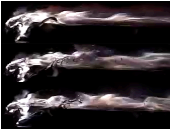
Fig. 8: Progression of a roll wave in the liquid layer during the zoomed in test at atmospheric pressure. Droplets can clearly be seen escaping the wave and entraining in the flow in the second and third frames. The second frame is 0.013 seconds after the first and the third frame is another 0.004 seconds after that.
