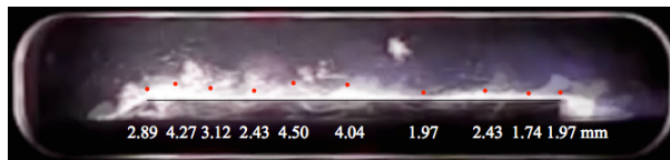
Fig. 14: Thickness of the optically bright region of the flame from the elevated pressure test. The height of the red dots above the black baseline is given in millimeters.
