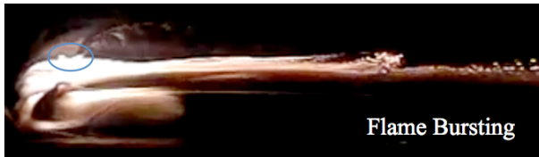
Fig. 9: Flame bursting at the very end of the atmospheric pressure test of blackened paraffin.
