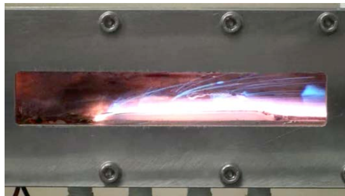
FIG. 7: Droplets entrained from the surface of paraffin burning with GOx from the video of Nakagawa et al. (2009).
