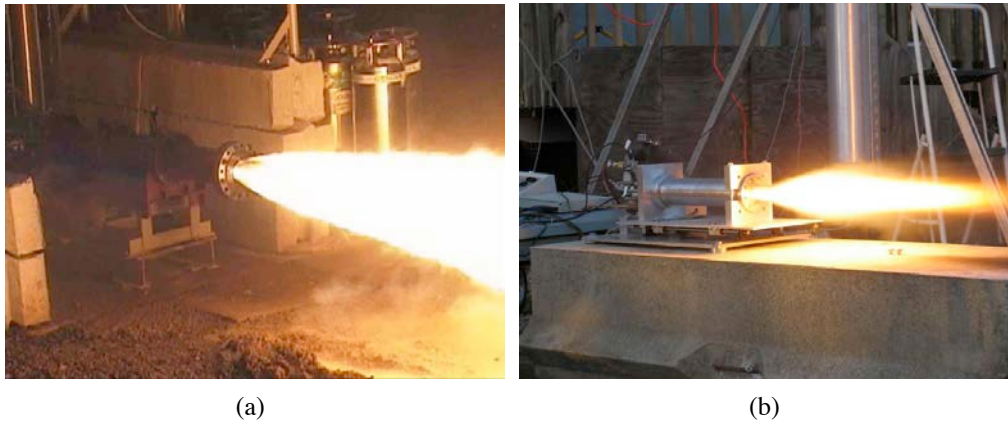
FIG. 9: SPG tests: (a) Scale-up test using liquid oxygen. Thrust is approximately 7000 lb, grain diameter is 10 in. with a 5:1 converging–diverging nozzle. (b) Small-scale test using nitrous oxide. Thrust is approximately 150 lb, grain diameter is 2.7 in. with a 3:1 converging–diverging nozzle.
