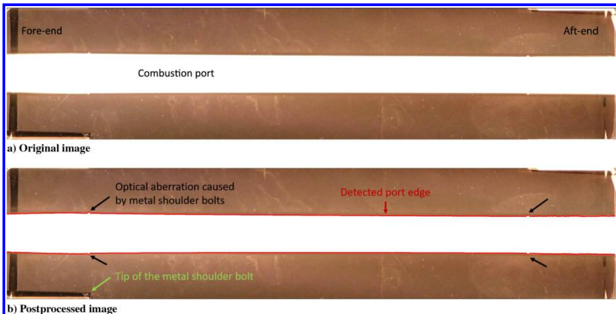
Fig. 2 Edge detection with ideal camera settings. The fuel port edge is resolved with a globally determined threshold and visible on the postprocessed image.
