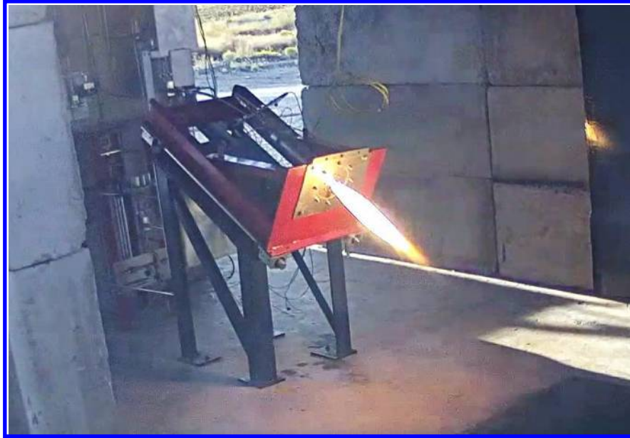
Figure 6. Image captured during static test firing with MON-3 oxidizer
