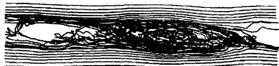
FIG. 21. Streamlines for tbl at tU/\delta_0 = 76.3 .
