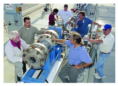
NASA Ames Research Center has tested forty 7.5-in.-dia. wax motors in its Hybrid Combustion Facility. Stanford and Ames have a joint hybrid r esearch program.
