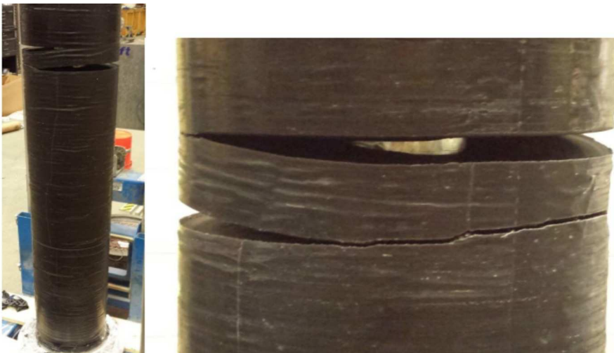
Full-scale paraffin fuel grain cast using incremental additions of paraffin wax wafers. Residual stresses arising from this method led to visible cracking of the grain.
