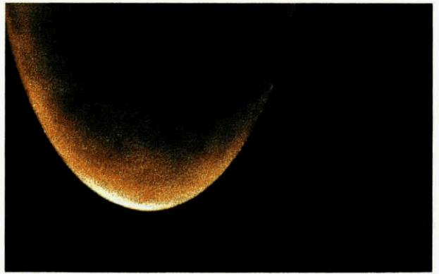
a) High tensile strength of the test water; no cavitation; V_\infty = 9,50 m/s \sigma = 0,69
