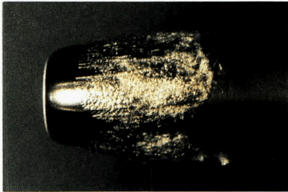
b) body size: 30 mm, \sigma = 0.26 , V_\infty = 11.0 m/s somewhat developed cavitation
