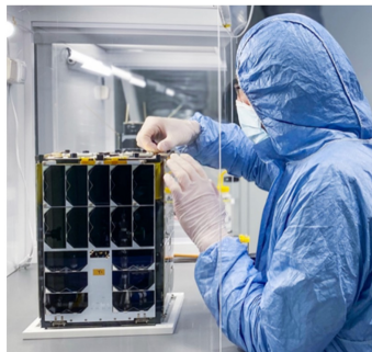
Advanced Composite Solar Sail System's, or ACS3's, 12-unit (12U) CubeSat spacecraft bus undergoing assembly and testing. The complete ACS3 spacecraft measures approximately 9 inches x 9 inches x 13 inches (23 centimeters x 23 centimeters x 34 centimeters), or about the size of a small microwave oven.
