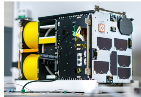
Advanced Composite Solar Sail System's, or ACS3's, 12-unit (12U) CubeSat spacecraft bus undergoing assembly and testing. The complete ACS3 spacecraft measures approximately 9 inches x 9 inches x 13 inches (23 centimeters x 23 centimeters x 34 centimeters), or about the size of a small microwave oven.
