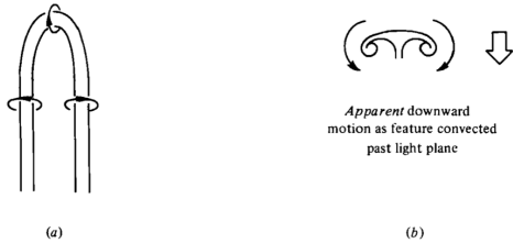
FIGURE 19. Views seen by camera as feature convected past light plane. (a) 45° downstream light plane; (b) 45° upstream light plane.
