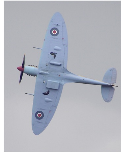
Figure 12.18 British Spitfire showing elliptic planform wing. Note the wing is formed from two ellipses of different minor axis. This shifts the major axis and center of lift forward.
