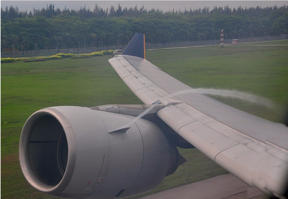
Figure 5.7 Condensation reveals the core of a chine vortex.
