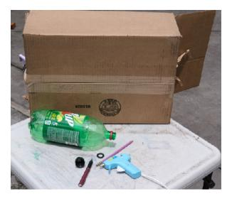
These are the materials we started with. Note the hot-glue gun is a "low-temp" type. This is important because if we damage the plastic bottle with heat it may blow up.
