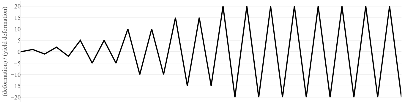
FIGURE 9 Load protocol applied in virtual quasi-static tests
