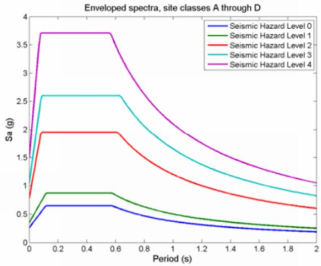
**Figure 6:** Design spectra obtained by enveloping over site classes A through D for the upper bound  $S_s$  and  $S_1$  values associated with each Seismic Hazard Level.
