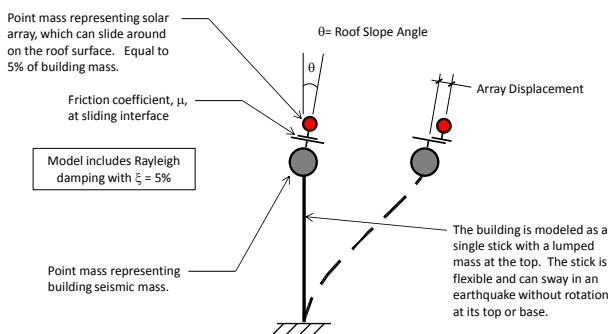
**Figure 10:** Schematic Representation of Analysis Model
