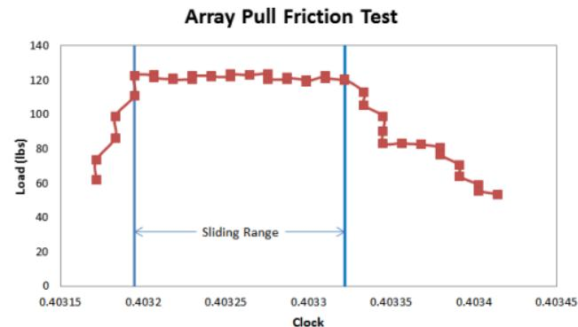
**Figure 9:** Sample test plot from example friction pull test of a PV array
