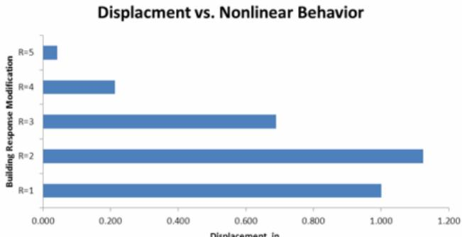
**Figure 15:** Horizontal displacement comparison at varying response modification coefficient values. Site Class A through D with slope at 1/4": 12". Normalized to R = 1
