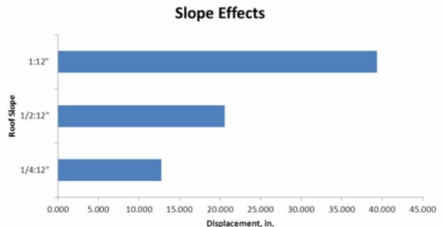
**Figure 17:** Horizontal displacement comparison at varying roof slopes. Site Class A through D with slope at 1/4": 12"
