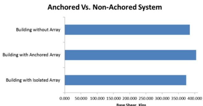
**Figure 16:** Building horizontal base shear comparison between anchored, non-anchored and building without array. Site Class A through D with slope at 1/4": 12"
