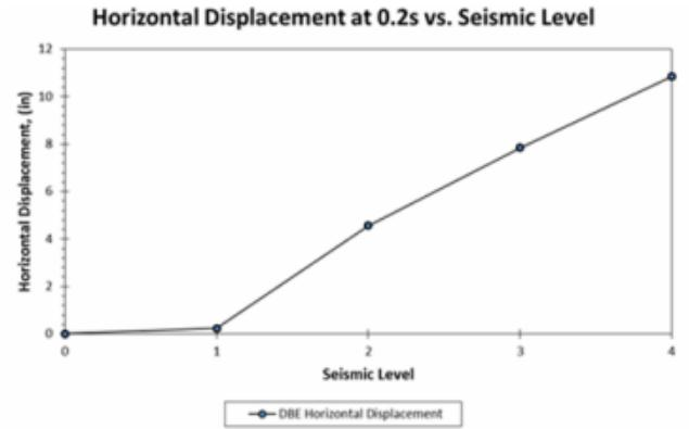
**Figure 14:** Displacement Occurrence Threshold Corresponding to Seismic Intensity Level
