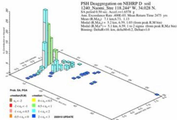
**Figure 12:** DBE Deaggregation for Example Site.
