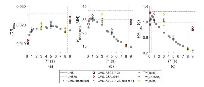
**Fig. 6.** Comparison of EDP results of theoretical and practical CMS procedures at MCE hazard level: (a) interstory drift ratio, (b) base shear, (c) roof acceleration.
