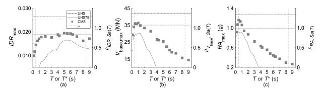
**Fig. 5.** EDP results of theoretical CMS procedure at MCE hazard level: (a) interstory drift ratio, (b) base shear, (c) roof acceleration. Values of EDP-Sa(T) correlation coefficients superimposed.
