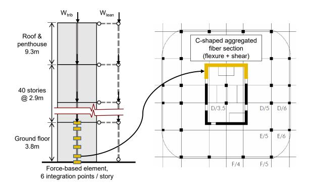
**Fig. 2.** Diagram of the case study building model, in elevation (left) and section (right). (Figure adapted from Zhong et al. (2021). Story plan view at right adapted from Moehle et al. (2011).)
