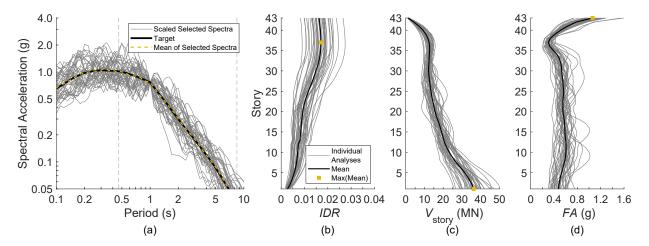
**Fig. 3.** Results of ground motion selection and nonlinear response history analysis for CMS target with  $T^* = 1s$ : (a) spectral target and individual selected spectra; (b)-(d) peak EDPs generated at each story.
