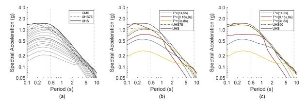
**Fig. 4.** CMS-based target spectra sets for different ground motion selection procedures: (a) theoretical CMS, (b) ASCE 7-22, (c) C&A-14. UHS-based spectra shown for reference.
