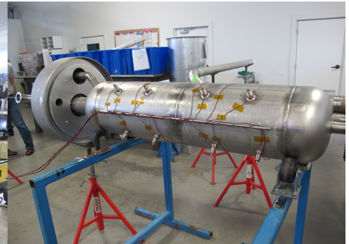
Thermocouples mounted to inner vessel
