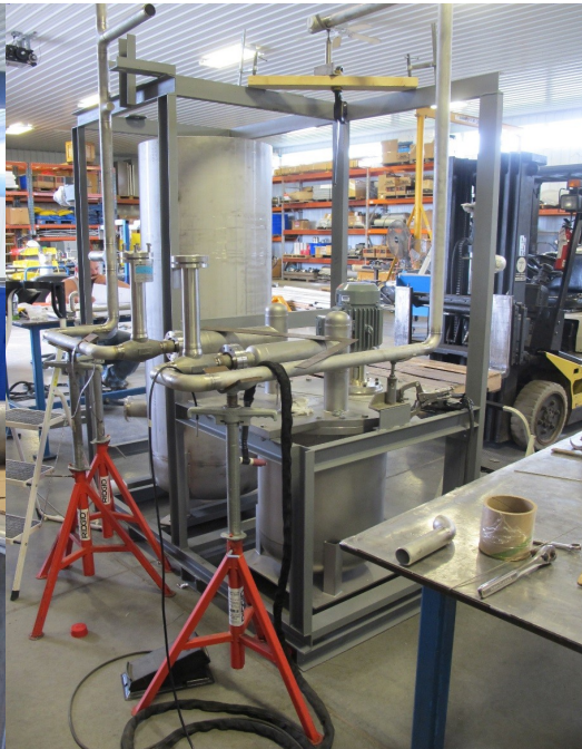
Filter skid frame assembly with pump mounted
