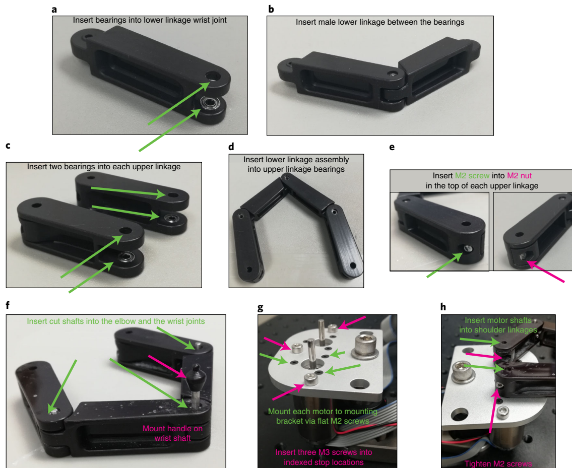
Fig. 2 | Detailed manipulandum assembly. a , For the lower linkage with pockets at one end, insert a ball bearing into each pocket, making sure to press firmly to insert fully. b , Insert the small end of the remaining lower linkage between the two bearings. When inserted correctly, the joint should rotate freely. c , For each (identical) upper linkage, insert a ball bearing into each pocket, making sure to insert fully. d , Take the free ends of the combined lower linkages and insert between the upper linkage ball bearings. e , Insert a button head M2 screw (from the outer side of linkage) into a thin M2 hex nut (pressed into the pocket in the inner side of the linkage) at the free end of each upper linkage. f , Insert one of the 12-mm cut shafts into each elbow joint and the 22-mm cut shaft into the wrist joint. Press the plastic handle onto the top of the wrist joint shaft. g , Affix each motor to the bottom of the mounting bracket by matching the tapped M2 holes on the motor to the M2 bores on the bracket and inserting a flat M2 screw into each. Also insert M3 screws into each tapped hole in the bracket to serve as the indexed mechanical stops for the manipulandum workspace. h , Press the holes of the free end of the upper linkages onto the motor shafts. Secure each upper linkage by tightening the button head M2 screw.
