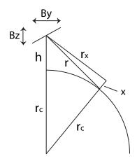
In this figure,  $r_c$  represents the local Earth radius of curvature, h is the satellite height, x is the topographic elevation at a point, r is the range to the reference sphere at the point,  $r_x$  is the range to the point at elevation, and By and Bz are the components of the baseline vector B. The parameters for the files we will use are:
